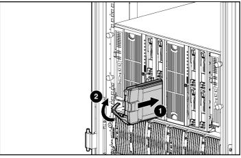
Figure 1-23: Installing a hot-plug SCSI hard drive
